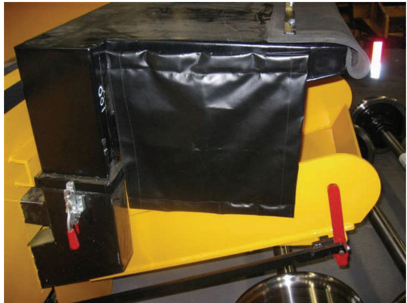
Dust Bin Cover Tarp 27299276 installed on CX Hammer.
