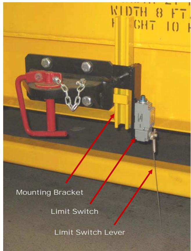
*The Crossing Alarm Switch Kit 98690014 includes a Mounting Bracket and Limit Switch that is attached to the front and back of the machine. The Limit Switch Lever ("whisker") extends downward to the track to detect the crossing.*
