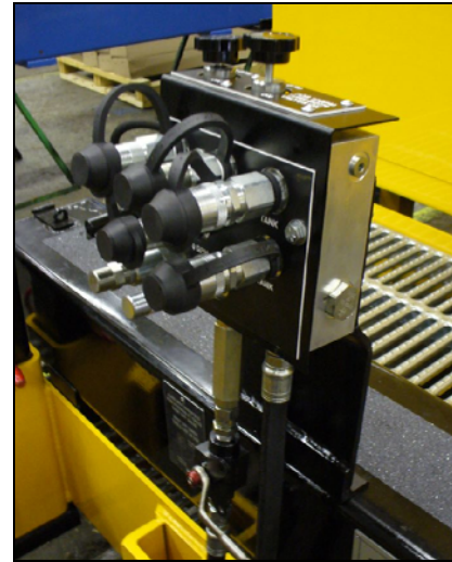
98330802 Hydraulic Tool Manifold Kit. The kit can also be used with other Nordco machines, including the NVCAR, NSCA and CGS in addition to the SP2R.
