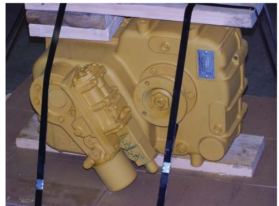
JD4664Y02EX: Calrk Transmission with Electric Coils
