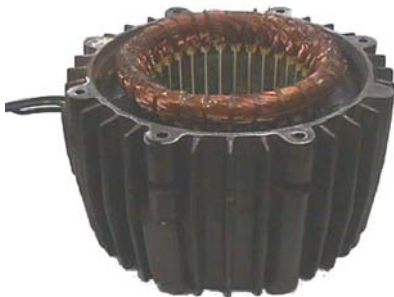
JE-1404809-0-01EX: Rebuilt Stator - Rewound and Notched
