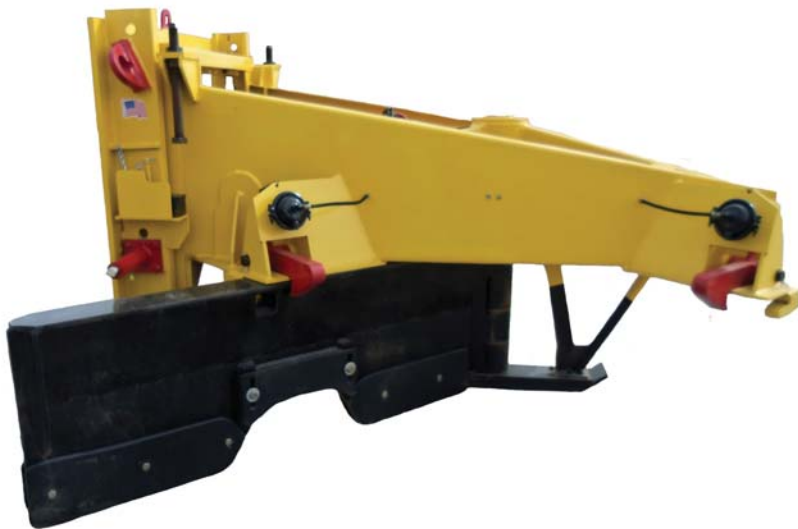
J9012626: Complete Rebuild of Single-Pass Ballast Plow with BTI Cutting Edges, Skid Plate, Wear Edges, and Rail Plates
