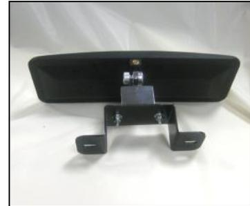
*96413602 Rearview Mirror Assembly Kit. Mirrors shown front and back, assembled to mounting bracket.*
