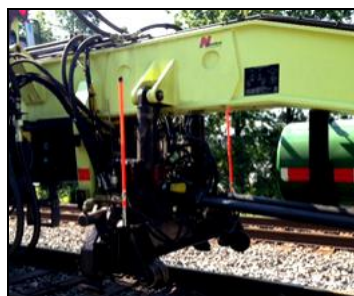
Left: Diagram shows placement of rods on rail lift frame. Middle: Rail Lift Guides installed on TRIPP machine. Above: 98760136 Rail Lift Guide Kit components.
