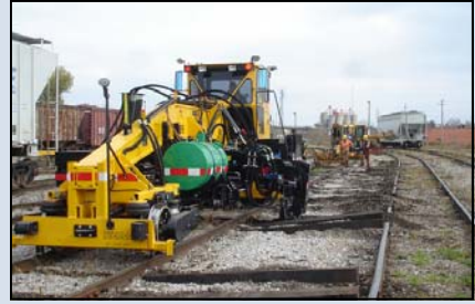
Service Schools are available for a wide range of Nordco machines, including the TRIPP Tie Exchanger.
