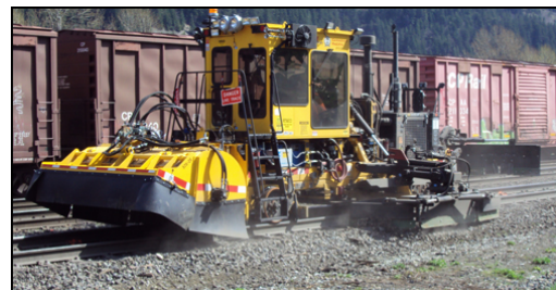
Nordco M7 Ballast Regulator.
