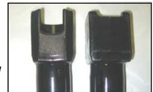
Curve Block (left) and Standard Anvil Sleeve.
