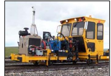
*Spring Clip Applicator, one of several Nordco machines that can use the Foot Switch Mounting Bracket Kit.*
