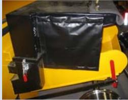
**27299276 CX Dust Bin Cover Tarp:** For all CX Hammers with Dust Suction Bulk Loader. Limits dust and debris entering the cab, improves efficiency of cab dust system. Easy installation, attaches with magnets, no special hardware required. Lift tarp for side access to chute. Two required per machine.
