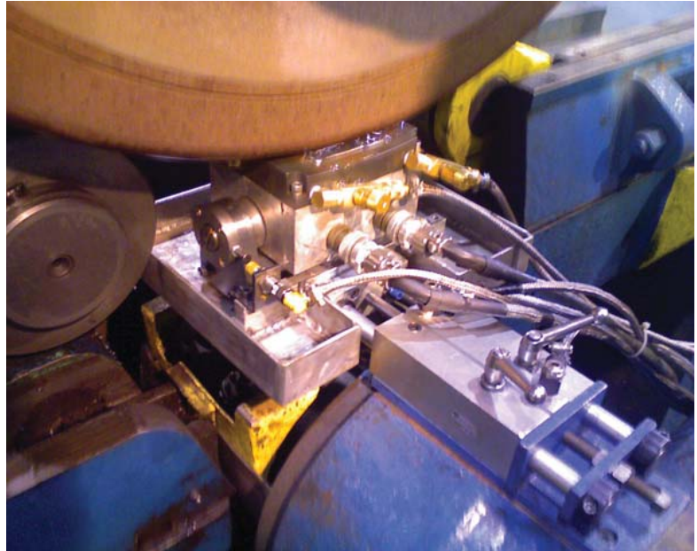
Inspection test head mounted on an underfloor profiling machine
