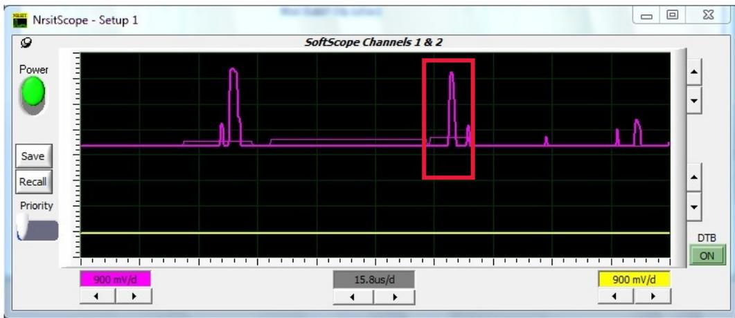
5. Tighten the Axel Shaft Collars while looking at the SoftScope to verify the peak does not drop.
