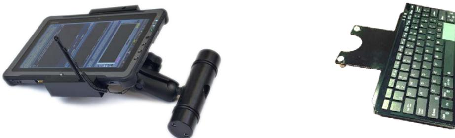
4. The Getac F110 tablet operates wirelessly so no further installation or hookup is required. In extreme heat operation,  $>90^{\circ}\text{F}$  ( $32^{\circ}\text{C}$ ), it is recommended to use a wired Ethernet connection by attaching an Ethernet cable to the relevant port on the F110 and the Ethernet connector located below the DSP housing on the OnePass. Follow the instructions from section 3.5.4 to setup the wired connection on the tablet.
