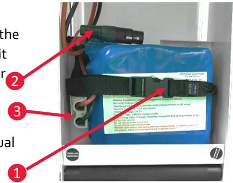
For testing applications that require air shipment of the OnePass, a Ni-Mh (Nickel-Metal Hydride) battery option is available (see image below and check Accessories and Add-Ons List at the end of this manual for part numbers). To charge the Ni-Mh battery:
