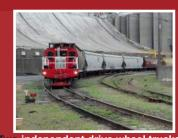
Two independent drive wheel trucks supported on rotating bearings with eight 16" AAR profile guide wheels. ABS & traction assist provide more control while reducing maintenance
