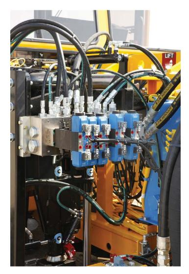
Easy access to the hydraulic fittings makes it simple and fast to replace hoses.
