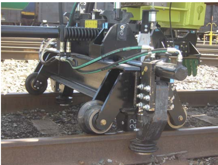
Rail jacks raise the rail while the gripper assembly inserts or removes the tie.
