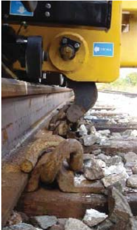
The included digital roller gauger allows gauging and spiking with one machine.
