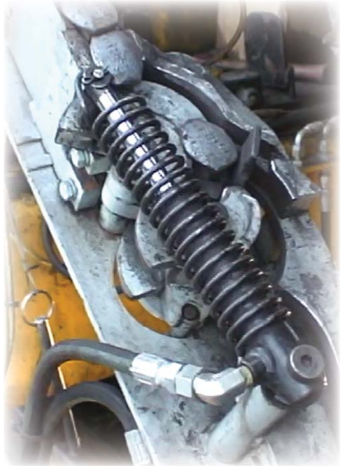
Orienter mechanism ensures that spikes are positioned correctly before entering the workhead.
