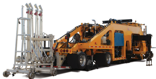
The RST-1000 features an easy-to-deploy TRIAD Reference System
