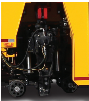
MultiClamp efficiently allows the RST-1000 to transition easily from RoadMode to RailMode.
