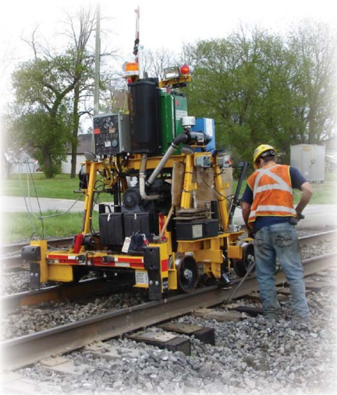
The Auto Lift can operate in both single and dual operator mode.
