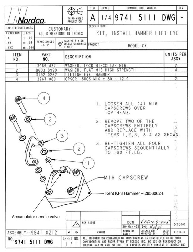
Figure 2 KF3 Lifting Eye Kit – 98410212 (CX Hammer and Model SS-B Spiking Machines)
