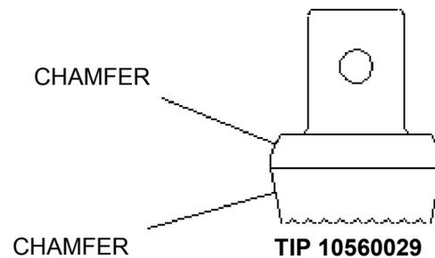
In addition, a solid drive pin, **p/n 53644000**, has replaced the roll pin, **p/n 53643950** which had been used to attach the tip to the anvil extension. This solid pin will eliminate reported problems with pin breakage. Since the solid pin "bites" into the anvil tip when installed, pin movement problems will be eliminated as well. **Anvil Tip p/n 10560029 will include one 53644000 pin.**
