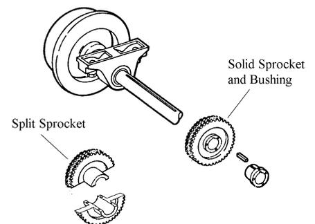
The following replacement axle assemblies have also been changed to incorporate the split sprocket:
