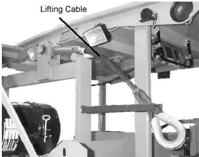
**Lifting Cable Installation**
