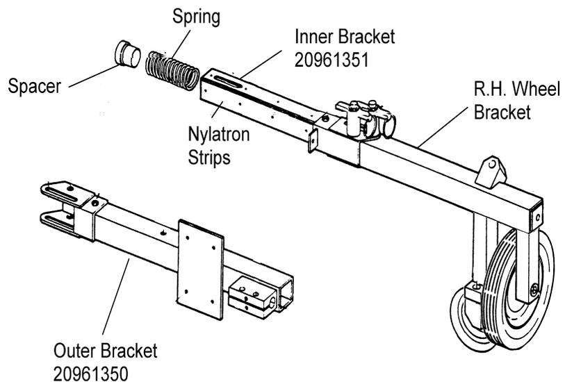
If the Nylatron strips require replacement, you do not need to return the entire Trak-Inspector. Only the inner bracket needs to be returned to NORDCO for repair.
