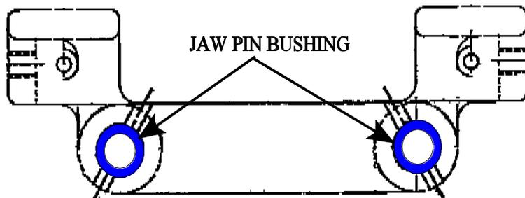
The steel bushing will wear longer than the bronze bushing in the 2135 8982 Jaw Mounting Assembly used on the Hydra-Hammer.
