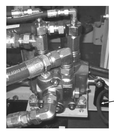
4000 PSI Propel Valve Note angled actuator rod.
