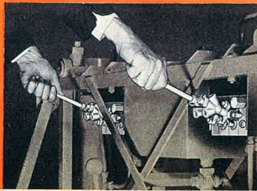
With both control levers pulled upward, oil is admitted to the bottom of the cylinders and the rams move upward.
