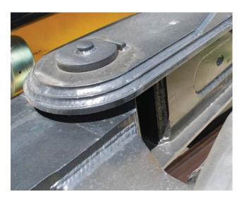
Breakaway boom joint protects boom by rotating backward when encountering an immoveable object.
