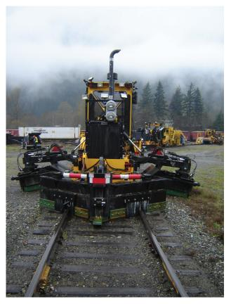
The operator-controlled positioning of wings, plows, and brooms allows for precise ballast sculpting and profiling.
