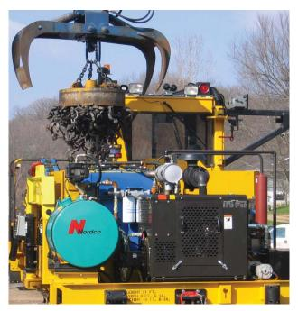
The bulk anchor bin is easily loaded, using either external magnet drops or the optional integrated boom and winch.
