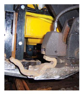
The anchor holders hold anchors firmly in place until the anchor application cycle is started.
