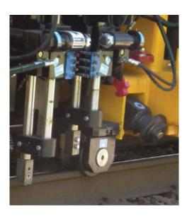
The pusher and scraper tools work in unison to remove anchors cleanly and completely.
