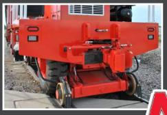
Wide range AAR sliding couplers are air released and hydraulically positioned.
