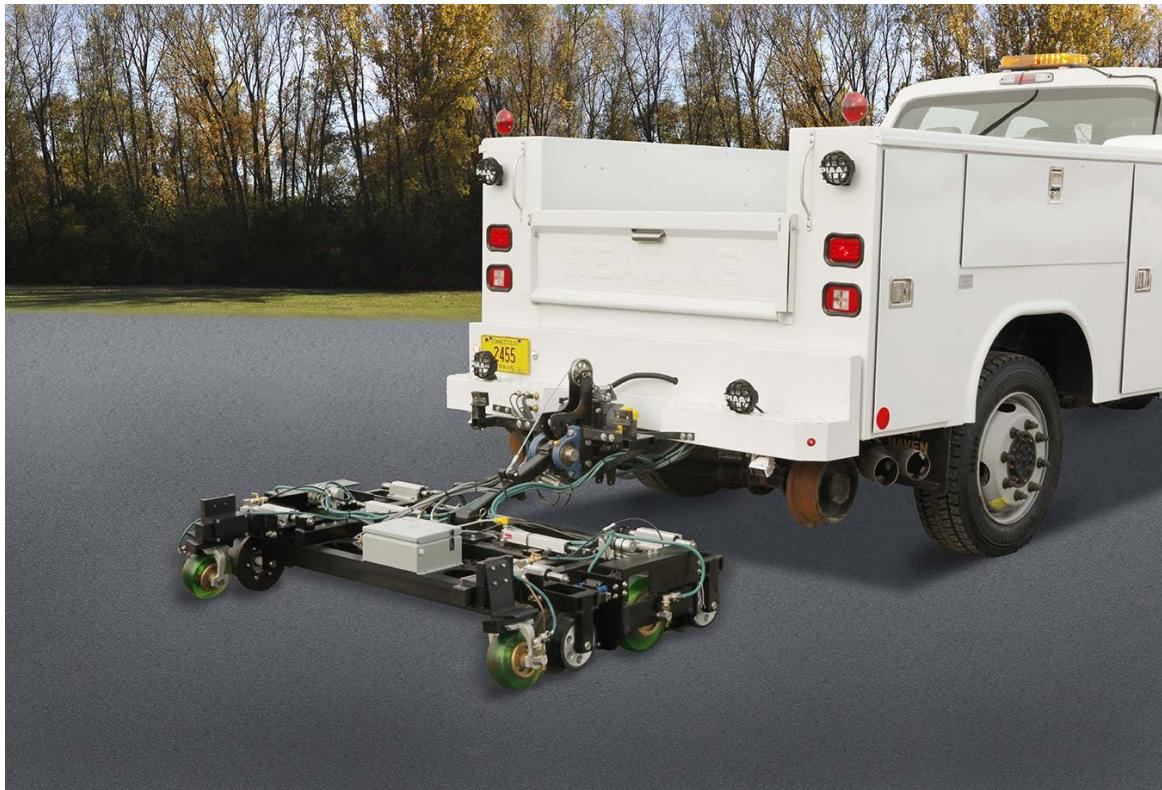
Nordco's is pleased to announce the new Flex rail flaw detection, featuring a hitch-mounted inspection carriage with patented XL9-11 wheel probes (including 11 inspection transducers), digital signal processing, and on-board Run-on-Run software.
