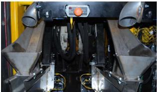
The spike tray forces the spike to drop vertically in the Orienter guide rail
