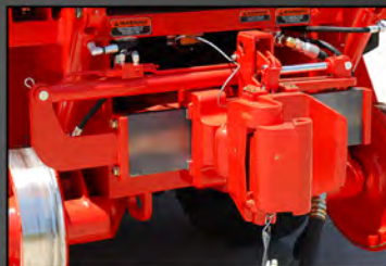
Wide range AAR sliding couplers are air released and hydraulically positioned to improve pulling performance on curves and grades.
