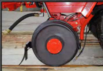
Powerful air knife increases capacities up to 50% in adverse weather.
