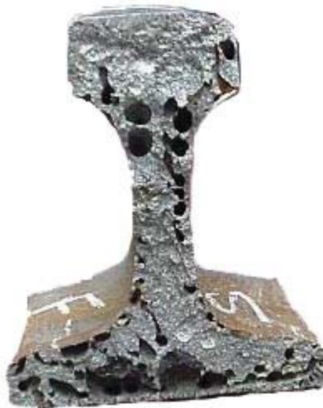
Thermite weld showing severe porosity
