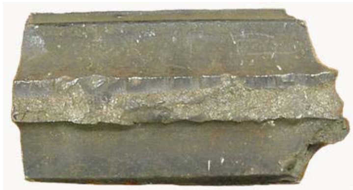
Head and web separation showing progression into the web.
