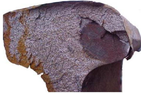
Detail Fracture Originating from a Visible Shell
