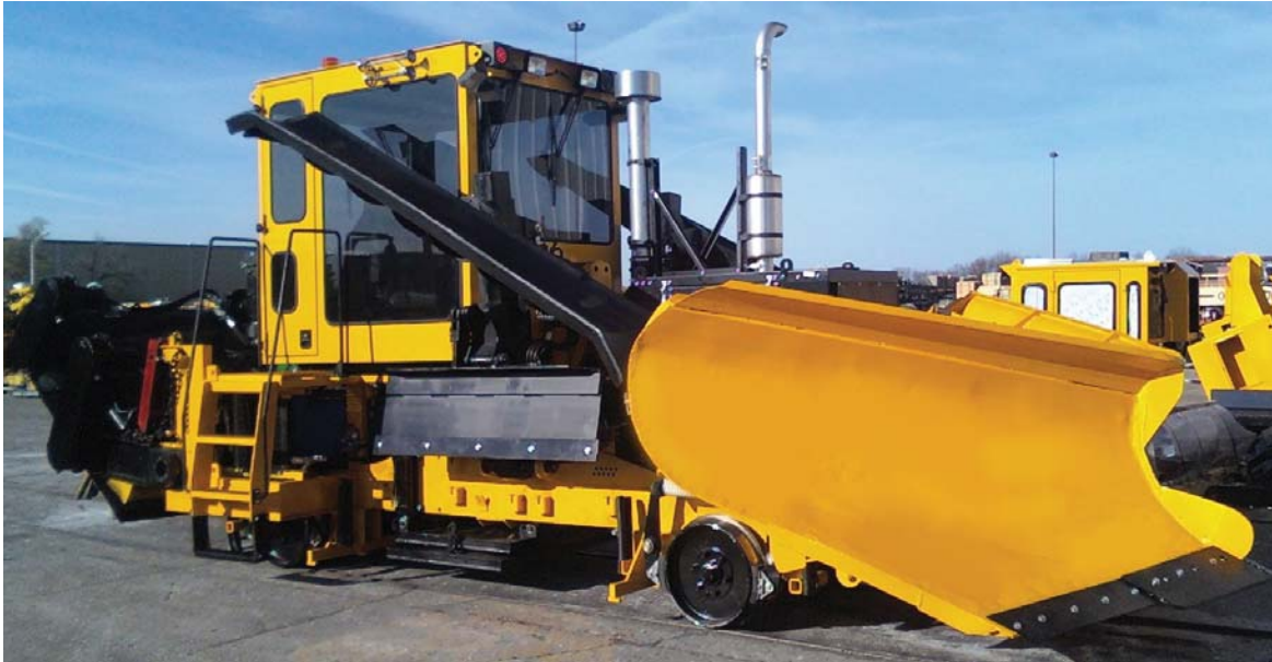
Ballast Regulator after rebuild
