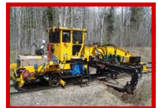
Nordco TRIPP Tie Exchanger
