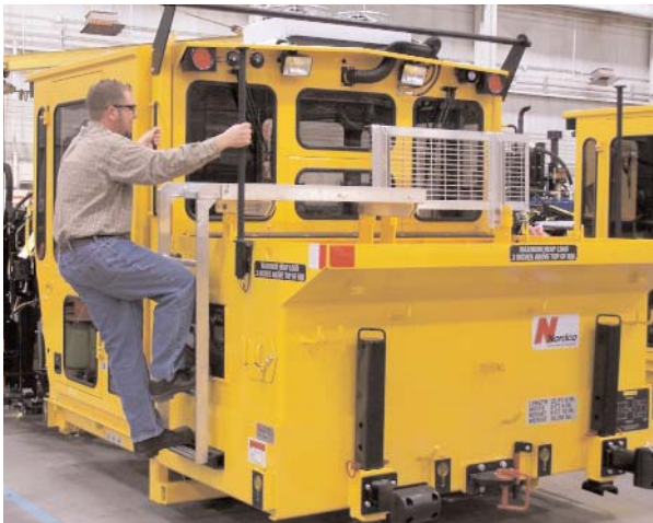
The aluminum ladder and handrail provide a stable, three-point-contact method of getting to or from the Walkway.
