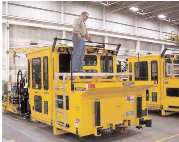
The Bulkloader Walkway provides a sturdy platform for accessing the top of the cab or the bulkloader bin.
