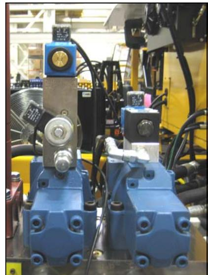
*Valve stack following installation of 98760289 Insertion Speed Control Kit.*
