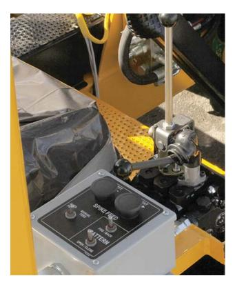
Operators control how spikes feed into the driving guns - selecting between manual or automatic mode.
