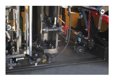
The gauger assembly allows rapid, yet extremely accurate, track setting at the correct gauge.
