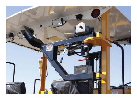
Included boom and winch make it easy to load kegs onto the rear deck.
