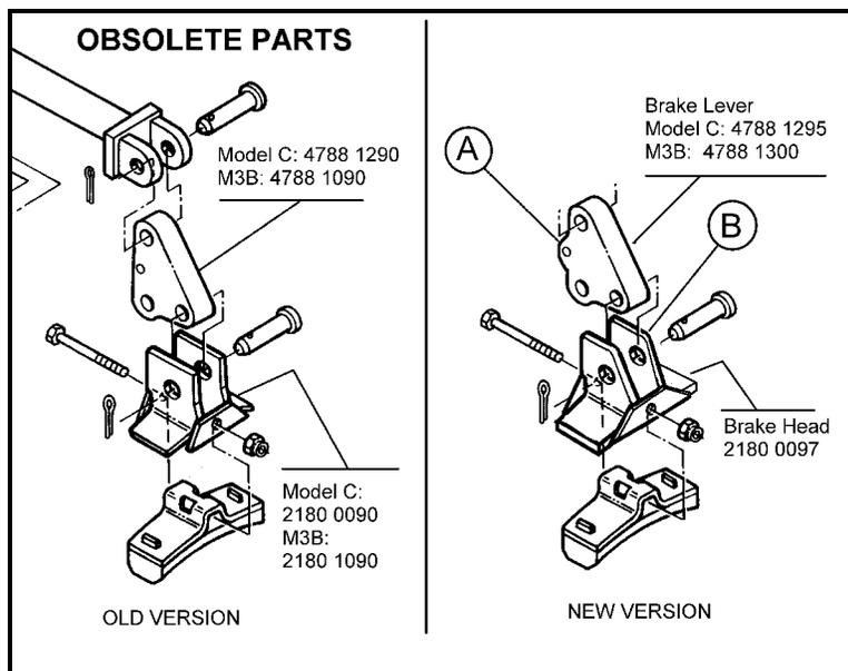
The primary changes in design were at points "A" and "B" in the new version shown. Both became more rounded to provide a better fit.
