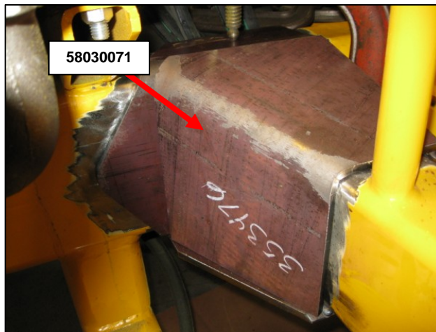
Figure 3 LH Tie-down Reinforcing Plate 56300071
