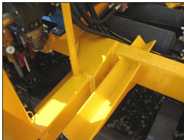
Figure 4 Completed Frame Reinforcement
