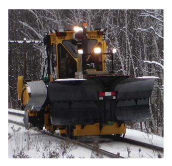
Plow blades move up and lock into travel mode to allow up to 35 mph travel speeds.
