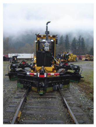
The operator-controlled positioning of wings, plows, and brooms allows for precise ballast sculpting and profiling.
