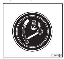
● The engine temperature gauge pointer should remain in the green sector most of the time. It should rarely enter the yellow-green sector. If the pointer enters the orange sector, the engine is overheating. Turn off and establish the cause from the Diagnosis Chart (see 7.1).
