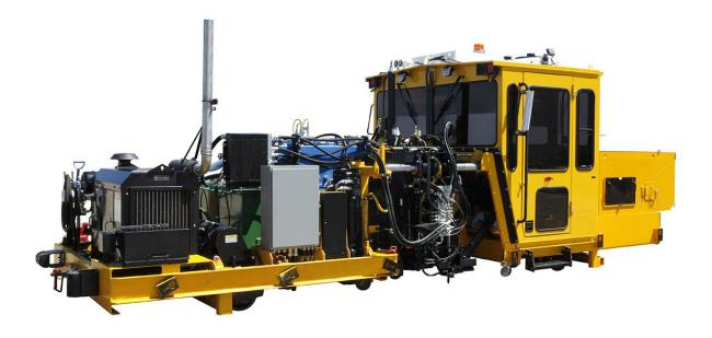
Nordco Inc.'s new CANbus-controlled production spike driver – SE Hammer – offers both productivity improvements as well as increased operator controls.
