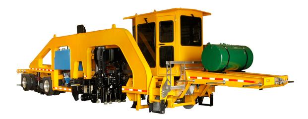
Nordco Inc.'s road-ready mobile tamper finally offers the railroad industry a revolutionary new reactive tamping solution that marries high production with unprecedented mobility.
